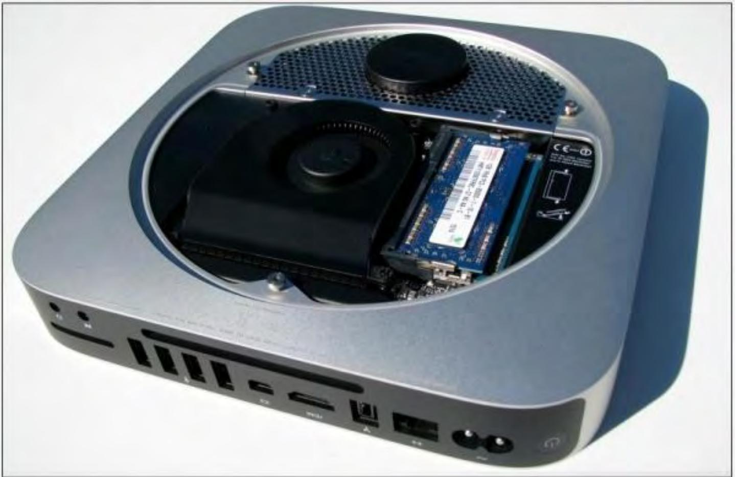
Figure 1. The Mac mini offers a removable panel for accessing its RAM chips.
