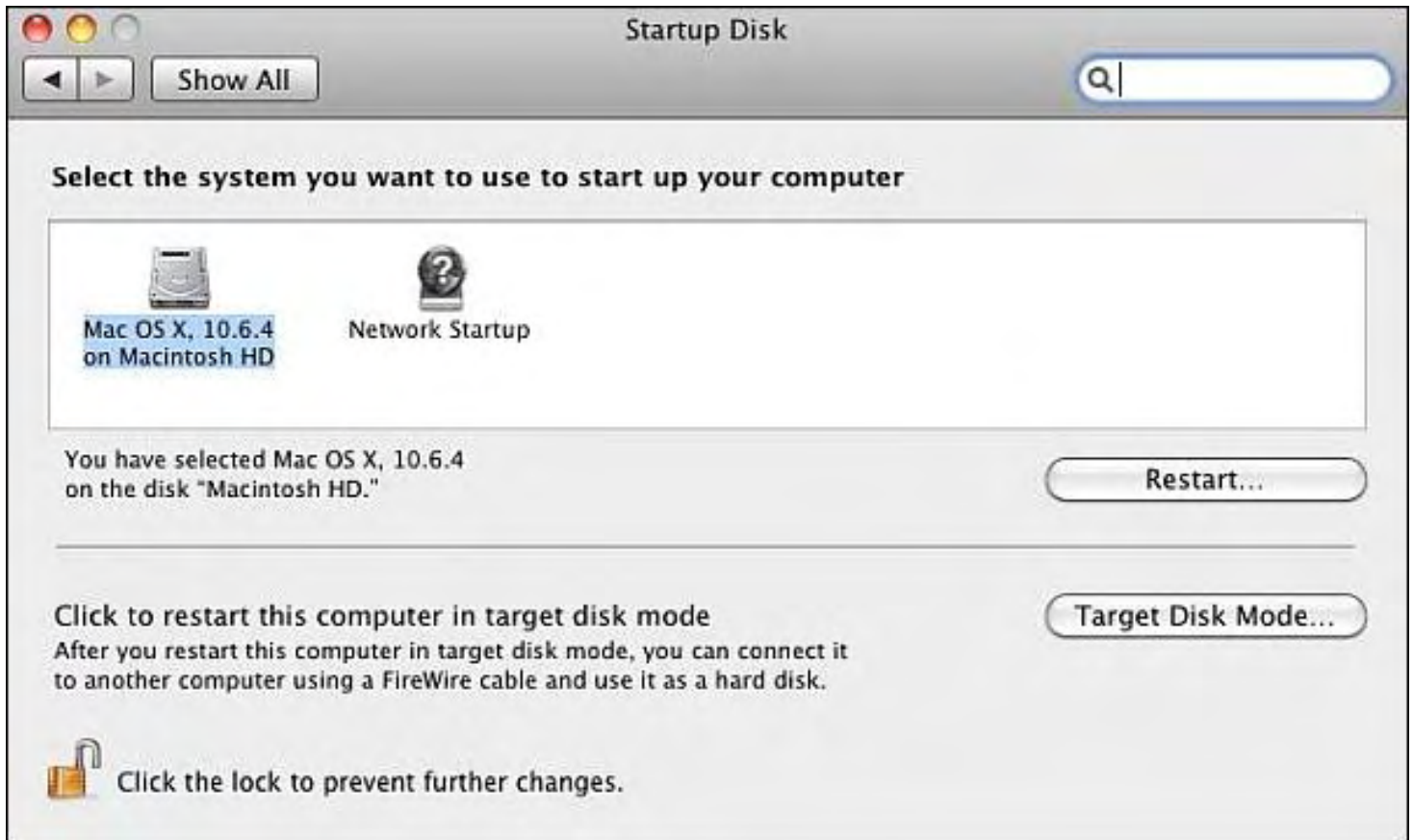
Figure 4. The Target disk Mode button lets you treat a Macintosh as an external hard disk.
