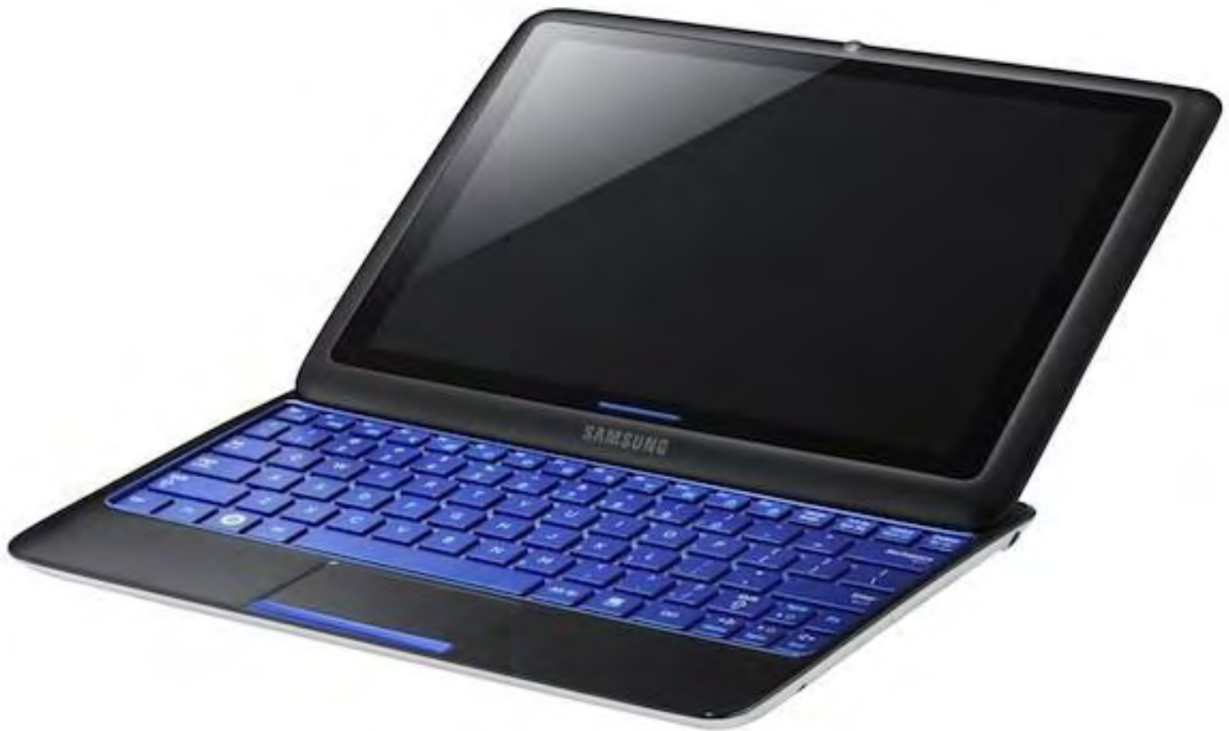
Figure 2. Samsung's Sliding PC lets you turn a tablet into a laptop with a slide out keyboard.
