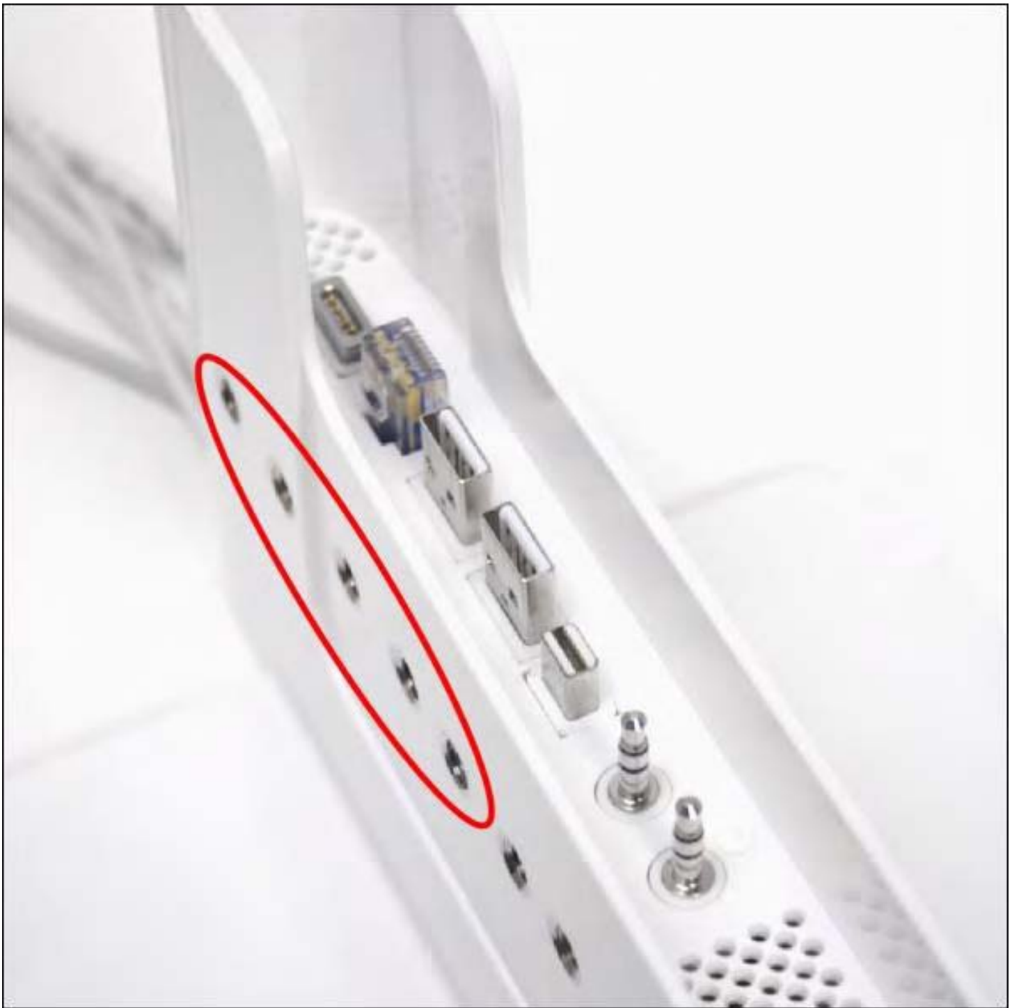
Figure 2. Some assembly is required with Henge Docks' docking stations. For each port to be used, the corresponding cable needs to be installed from the docking station's underside into the corresponding void, then secured with a set-screw (red) so that the connector properly aligns with and inserts into the computer's corresponding port without damaging the port.
