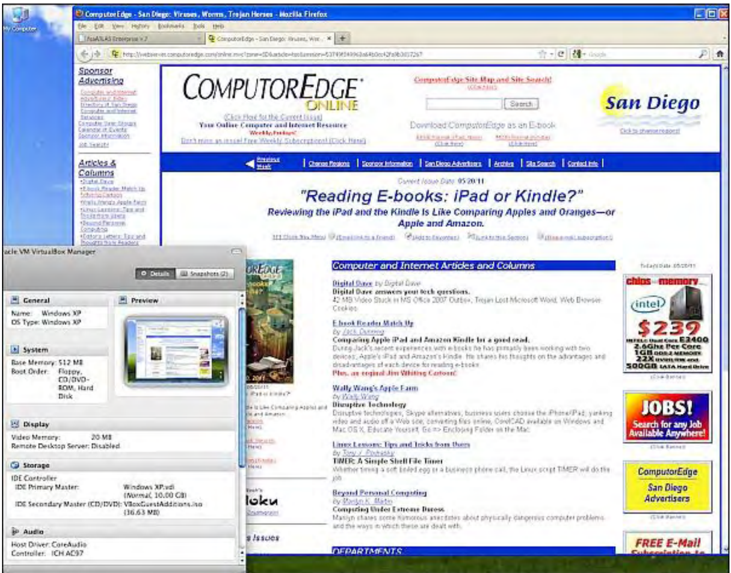
Figure 2. A VM can be operationally defined as a set of conditions (configuration) for running an additional OS alongside the boot OS and for displaying the other OS in a window that the user interacts with. In this screen capture of Windows XP in a VM, the configuration appears in the window at the lower left corner.
