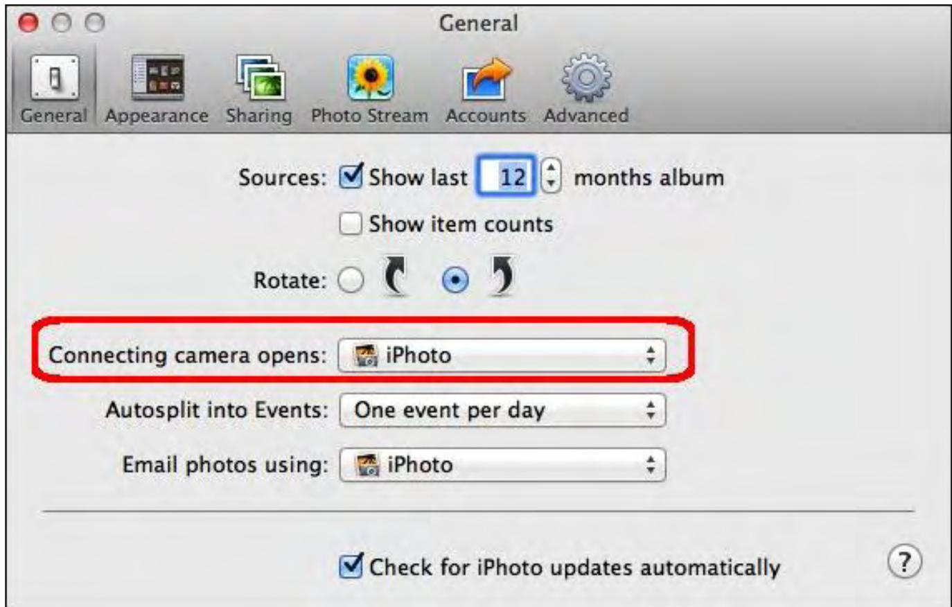
Figure 4. Defining the default program to load when you connect a camera to a Mac.
