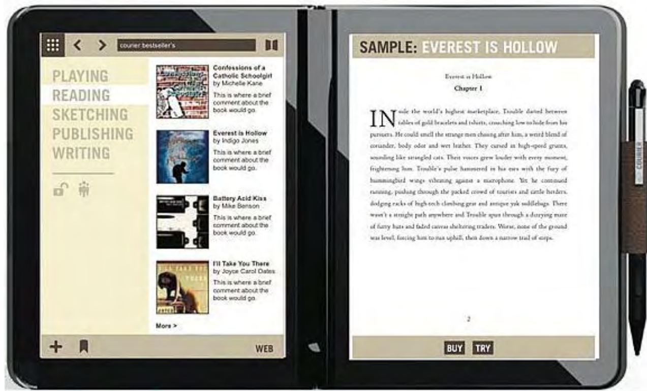
Figure 1. The Courier tablet would have displayed dual screens hinged together like a book.
