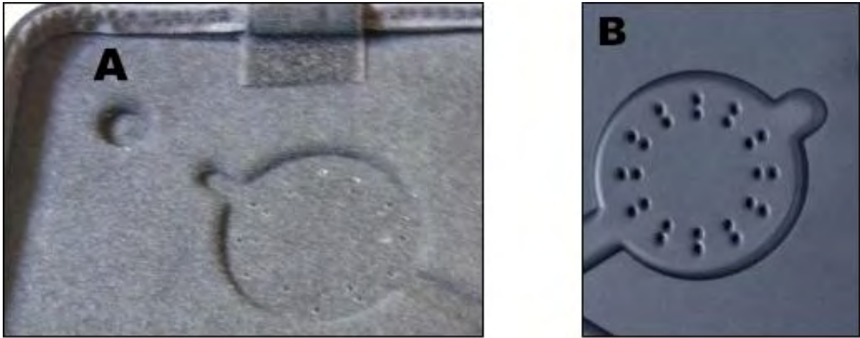
Figure 2. Passive cooling is provided by holes arranged in a recessed array (shown from the inside in A, from the outside in B) built into the Ventilator case's bottom part. To close these venting holes, the user inserts an orange seal with a velcro underside into the recess.
