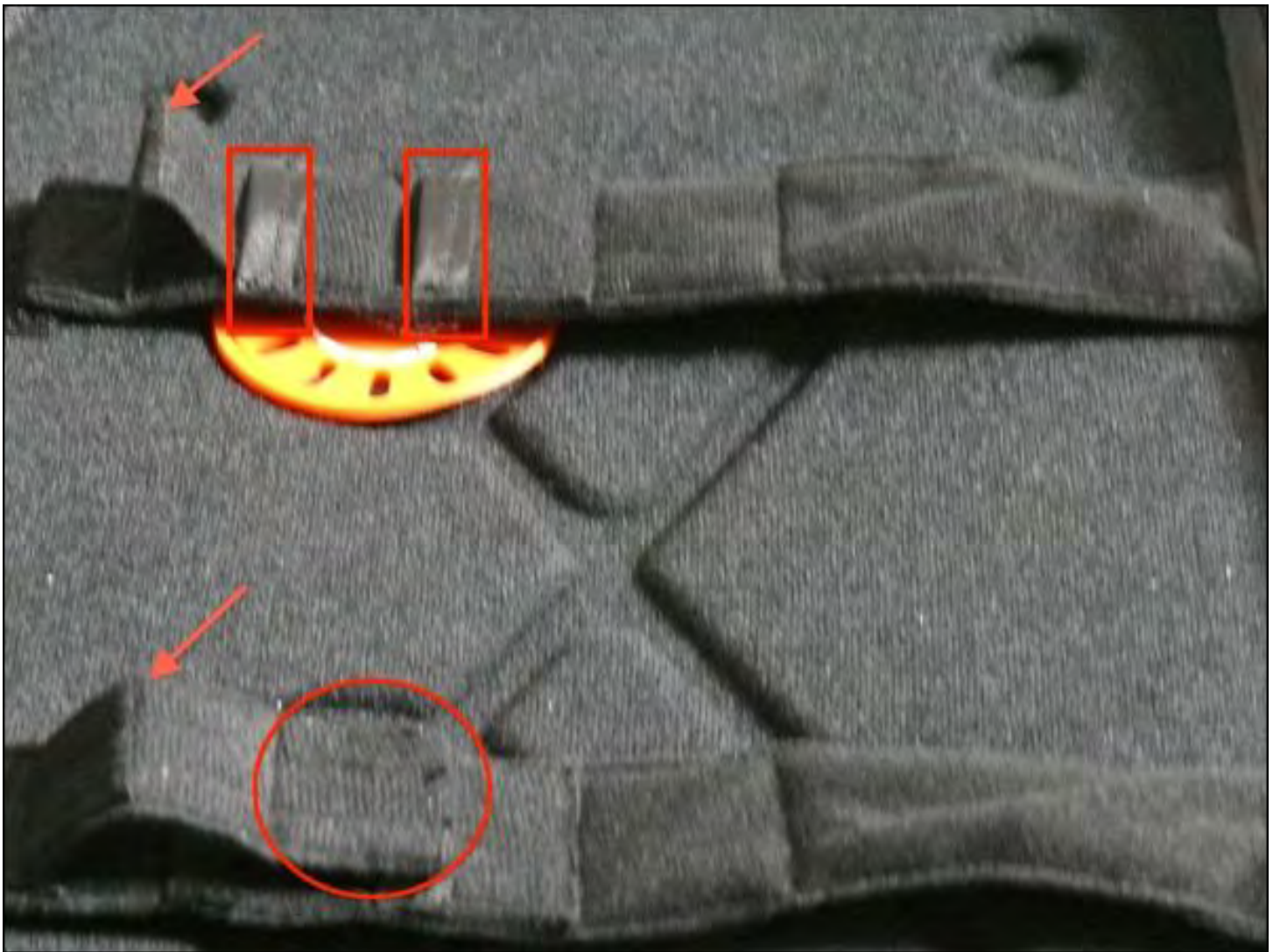
Figure 3. Passive cooling also is provided by two sturdy wedges (aka "risers"; red arrows) which are fabric strips (red circle) that, when inserted into one of two pockets (red rectangles) in each strip, prop up the screen end of the computer. This allows chassis heat to vent (grey arrows in Figure 1A) and cool air to flow under the chassis.
