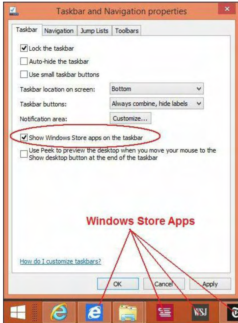
Figure 1. Checked by default, "Show Windows Store app on the taskbar" adds running Modern apps to the Taskbar and the Taskbar to the Modern interface screen.
