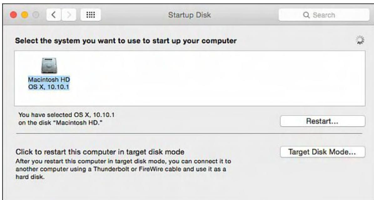
Figure 13. Target Disk Mode lets you reboot a Macintosh without the interference of OS X.
